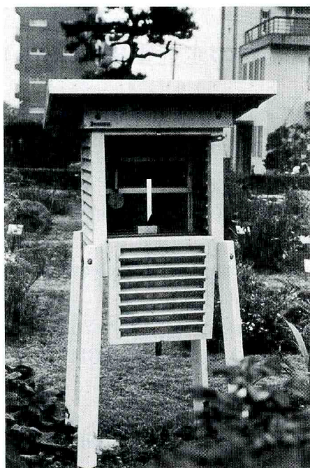
Fig. 1. A slide is setting in the instrument shelter, arrow points to the slide holder.
